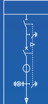
BME-08 Current & Voltage Measurement Cubicle With LBS
